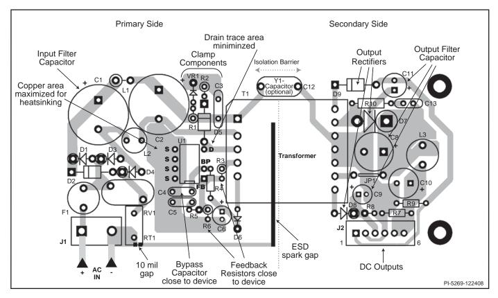
Figure 5. PCB Layout Example.
