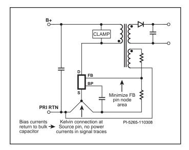
Figure 6. Schematic Representation of Recommended Layout Without External Bias.
