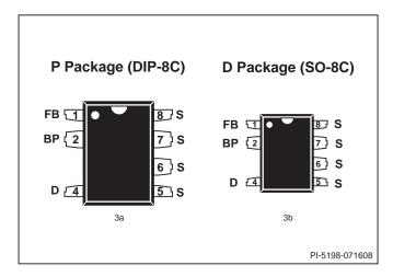
Figure 3. Pin Configuration.
