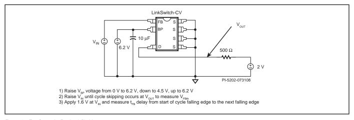
Figure 19. Test Set-up for Feedback Pin Measurements.
