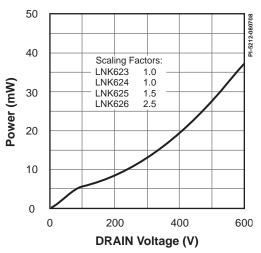
Figure 18. Drain Capacitance Power.
