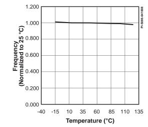
Figure 13. Output Frequency vs, Temperature.
