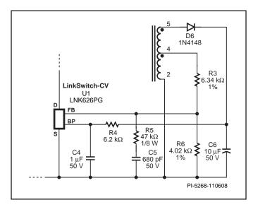
Figure 12. RC Network Across  $R_{\text{BOTTOM}}$  (R6) to Reduce Pulse Grouping.
