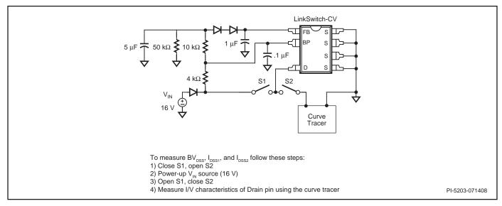
Figure 20. Test Set-up for Leakage and Breakdown Tests.
