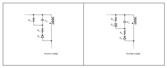
Figure 9. RCD Clamp, Low Power or Low Leakage Inductance Designs.
