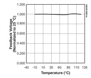
Figure 14. Feedback Voltage vs, Temperature.
