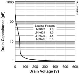
Figure 17.  $C_{\rm oss}$  vs. Drain Voltage.
