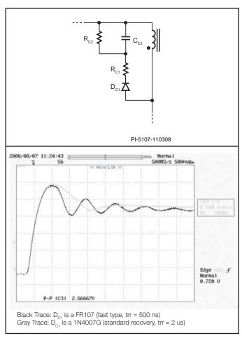
Figure 10. Effect of Clamp Diode on Feedback Pin Settling. Clamp Circuit (top). Feedback Pin Voltage (bottom).
