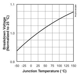
Figure 15. Breakdown vs. Temperature.
