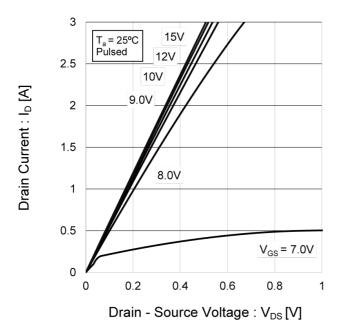
Fig.8 Typical Output Characteristics(II)
