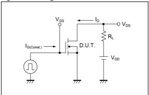
Fig.3-1 Avalanche Measurement Circuit
