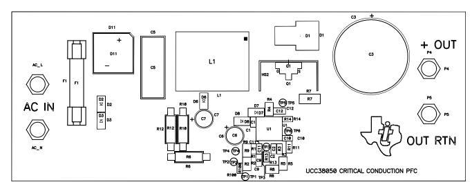
Figure 5. Reference Design Board Layout
