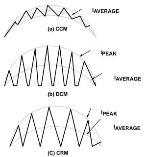
**Figure 2. PFC Inductor Current Profiles**
