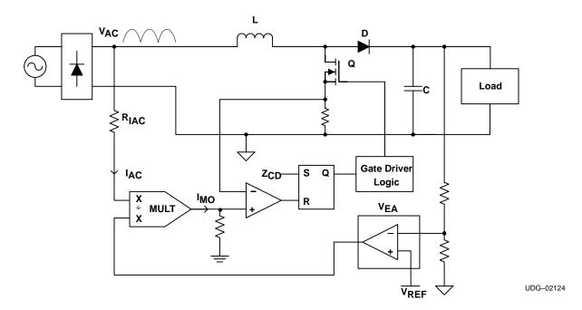
Figure 1. Basic Block Diagram of CRM Boost PFC
