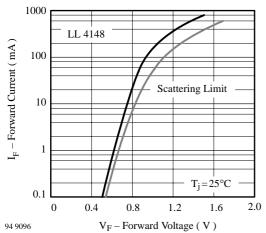
Figure 1. Forward Current vs. Forward Voltage
