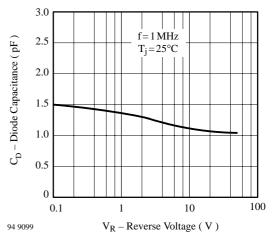
Figure 4. Diode Capacitance vs. Reverse Voltage
