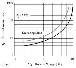
Figure 3. Reverse Current vs. Reverse Voltage
