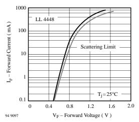
Figure 2. Forward Current vs. Forward Voltage
