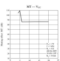
Supply voltage  $V_{CC}$  (V)
