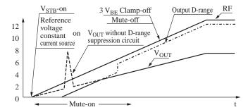
Image figure of output waveform, RF-pin waveform has exponential characteristics in actually.
