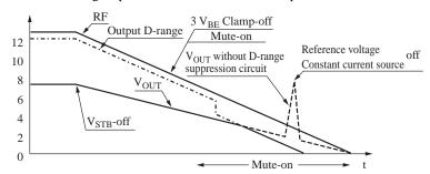
Image figure of output waveform, RF-pin waveform has exponential characteristics in actually.
