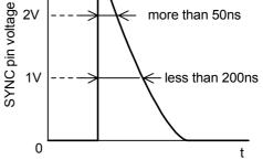
Fig.3 Condition for SYNC pin signal
