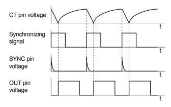
Fig.5 Timing chart of synchronized operation
