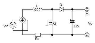
Fig.19 Boost converter circuit
