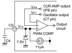
Fig.9 PWM comparator circuit
