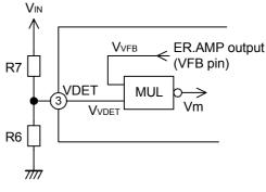
Fig.11 Multiplier circuit
