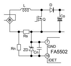
Fig.27 IDET pin protection (2)
