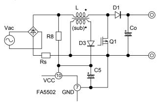
Fig.15 Vcc circuit (1)
