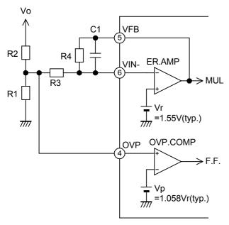
Fig.6 Voltage error amplifier and overvoltage limiting circuit
