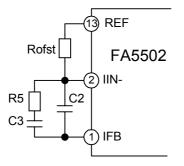
Fig.25 Connection of Rofst
