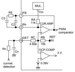
Fig.7 Current error amplifier and overcurrent limiting circuit
