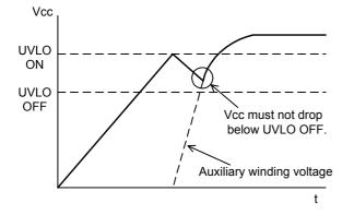
Fig.16 Vcc voltage at start up
