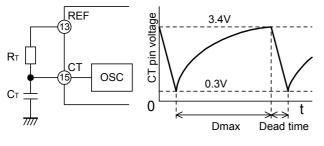
Fig.1 Oscillator circuit
