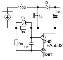
Fig.26 IDET pin protection (1)
