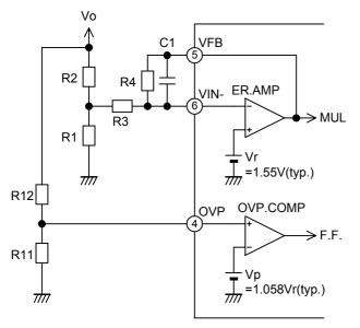
Fig.23 Independent setting of OVP limit
