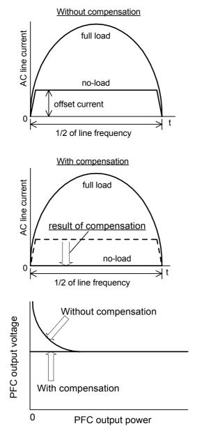
Fig.14 Operation outline of compensation circuit for light load
