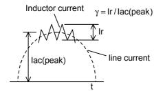
Fig.20 Outline of inductor and AC line current
