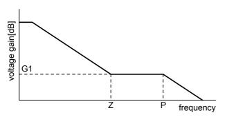
Fig.8 Voltage gain of CUR.AMP
