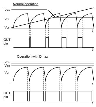
Fig.10 PWM comparator timing chart
