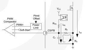
Figure 21. Current Sense and Feedback Circuits
