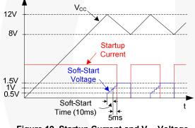
Figure 19. Startup Current and  $V_{CC}$  Voltage
