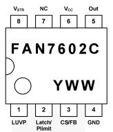
Figure 3. Pin Configuration (Top View)
