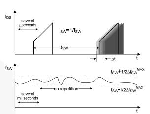
Figure 20. Frequency Fluctuation Waveform
