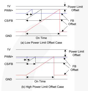
Figure 22. CS/FB Pin Voltage Waveforms
