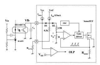
Figure 6. Pulse width modulation (PWM) circuit
