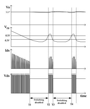
Figure 10. Waveforms of burst operation
