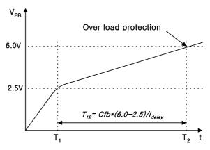
Figure 8. Over load protection
