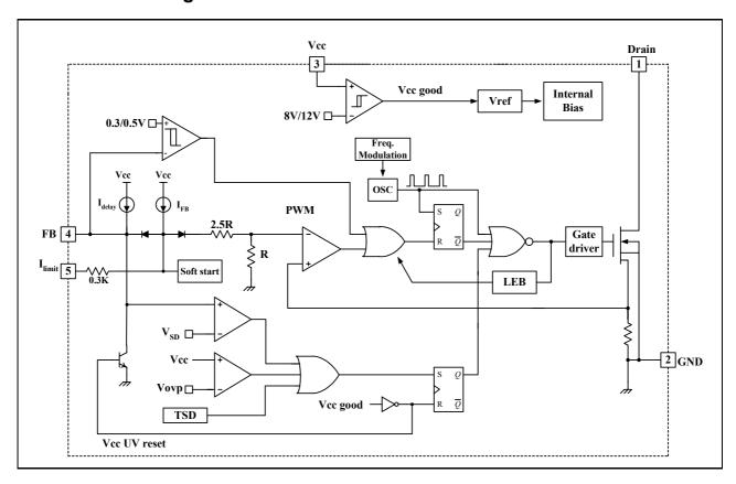
Figure 2. Functional Block Diagram of FSCM0765R
