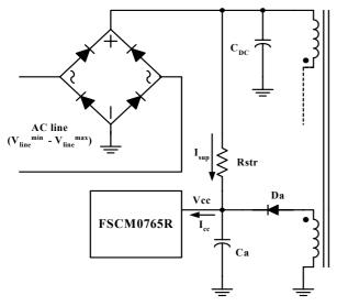
Figure 4. Startup circuit
