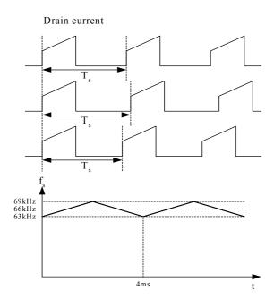
Figure 9. Frequency Modulation
