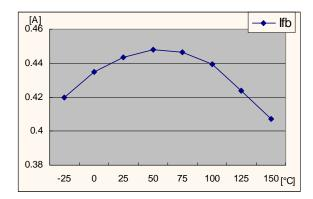
Fig 4. Feedback Source Current
