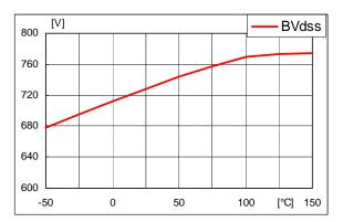
Fig 10. Breakdown vs. Temperature
