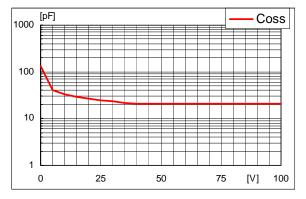
Fig 9. Coss vs. Drain Voltage
