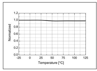
Figure 13. Burst-Mode High Threshold Voltage  $(V_{burh})$  vs.  $T_A$
