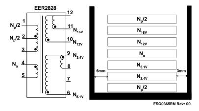
Figure 30. Transformer Schematic Diagram of FSQ0365RN
