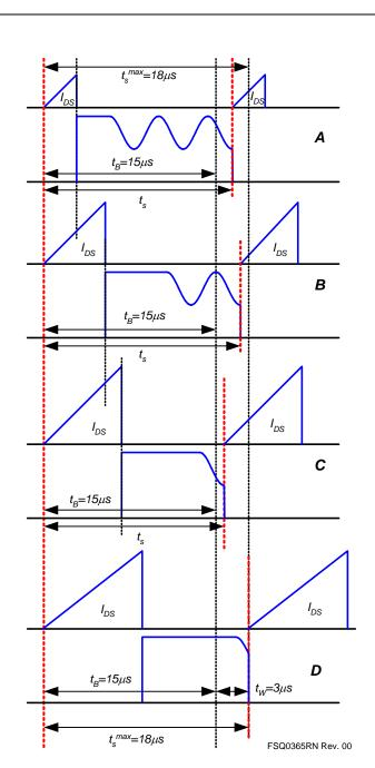
Figure 27. Valley Switching with Limited Frequency
