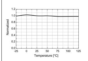
Figure 16. Sync High Threshold Voltage (V<sub>SH</sub>) vs. T<sub>A</sub>
