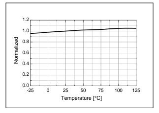
Figure 15. Peak Current Limit (I<sub>LIM</sub>) vs. T<sub>A</sub>
