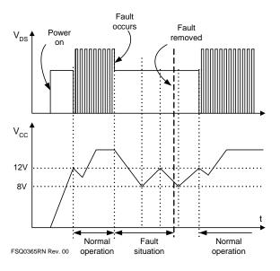
Figure 23. Auto Restart Protection Waveforms
