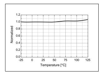
Figure 10. Blanking Time (t<sub>B</sub>) vs. T<sub>A</sub>
