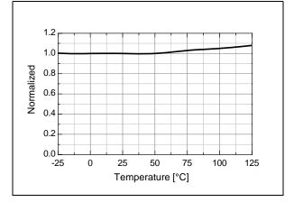
Figure 9. Maximum On Time ( $t_{ON.MAX}$ ) vs.  $T_A$
