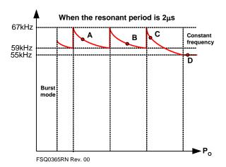
Figure 28. Switching Frequency Range
