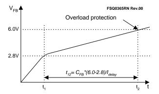
Figure 24. Overload Protection
