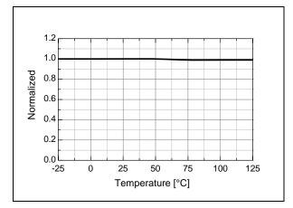
Figure 6. UVLO Stop Threshold Voltage ( $V_{STOP}$ ) vs.  $T_A$
