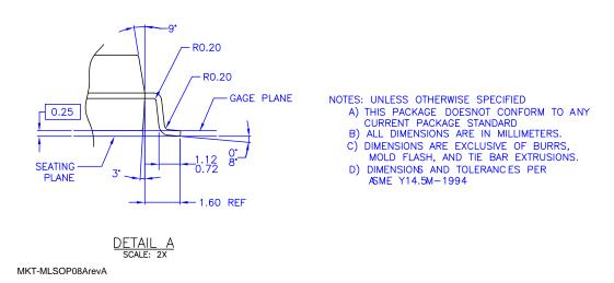
Figure 34. 8-Lead, LSOP Package
