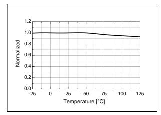
Figure 8. Initial Switching Frequency (f<sub>S</sub>) vs. T<sub>A</sub>
