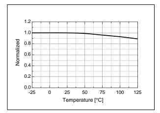
Figure 12. Shutdown Delay Current (I<sub>DELAY</sub>) vs. T<sub>A</sub>
