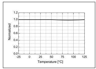
Figure 5. UVLO Start Threshold Voltage ( $V_{START}$ ) vs.  $T_A$
