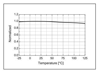
Figure 7. Start-up Charging Current (I<sub>CH</sub>) vs. T<sub>A</sub>
