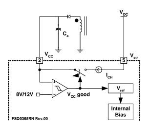
Figure 20. Start-up Circuit
