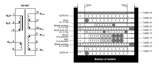
Figure 32. Transformer Schematic Diagram of FSQ311
