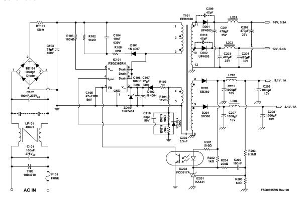
Figure 29. Demo Circuit of FSQ0365RN
