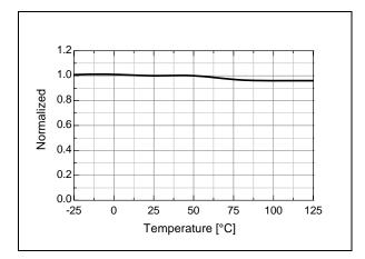
Figure 4. Operating Supply Current ( $I_{OP}$ ) vs.  $T_A$
