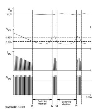
Figure 26. Waveforms of Burst Operation
