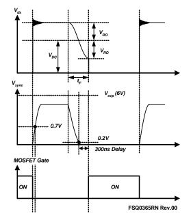
Figure 22. Valley Resonant Switching Waveforms
