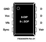
Figure 3. Pin Configuration (Top View)
