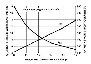
FIGURE 4. SHORT CIRCUIT WITHSTAND TIME
