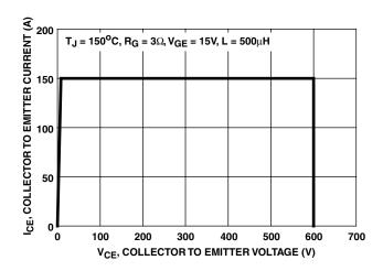
FIGURE 2. MINIMUM SWITCHING SAFE OPERATING AREA
