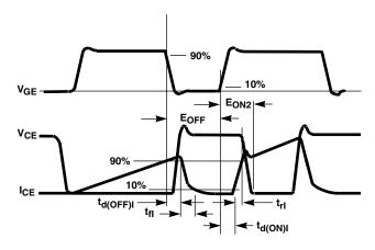
FIGURE 25. SWITCHING TEST WAVEFORMS
