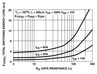
FIGURE 16. TOTAL SWITCHING LOSS vs GATE RESISTANCE
