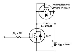
FIGURE 24. INDUCTIVE SWITCHING TEST CIRCUIT
