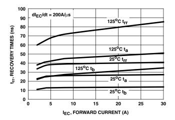
FIGURE 20. RECOVERY TIMES vs FORWARD CURRENT
