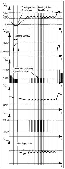
Figure 17 Signals in Active Burst Mode
