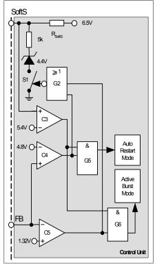
Figure 15 Adjustable Blanking Window
