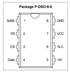
Figure 2 Pin Configuration P-DSO-8-8(top view)
