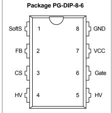
Figure 1 Pin Configuration PG-DIP-8-6(top view)
