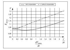
Figure 13 Overcurrent Shutdown
