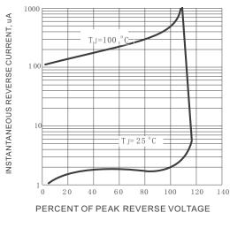
Fig.3 TYPICAL PEAK REVERSE CHARACTERISTICS
