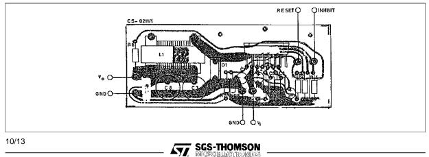
Figure 13 : Typical Application Circuit.
