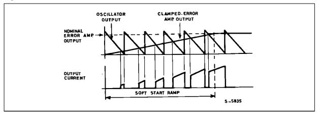
Figure 3 : Current Limiter Waveforms
