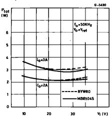
Figure 12 : Power Dissipation Derrating Curve.
