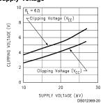
Clipping Voltage vs Supply Voltage
