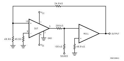
Test Circuit #2 (Note 3) (AC Electrical Test Circuit)
