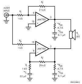
FIGURE 2. Bridged Amplifier Application Circuit
