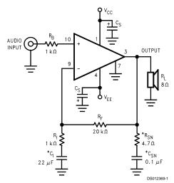
\*Optional components dependent upon specific design requirements. Refer to the External Components Description section for a component functional description.
