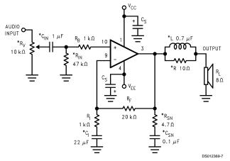
FIGURE 4. Auxillary Amplifier Application Circuit
