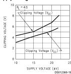
Clipping Voltage vs Supply Voltage
