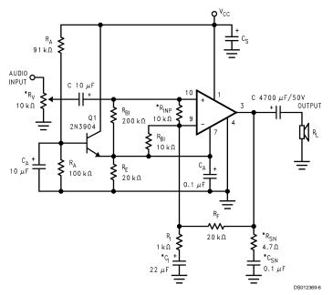
FIGURE 3. Single Supply Amplifier Application Circuit
