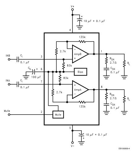
FIGURE 2. Test Circuit
