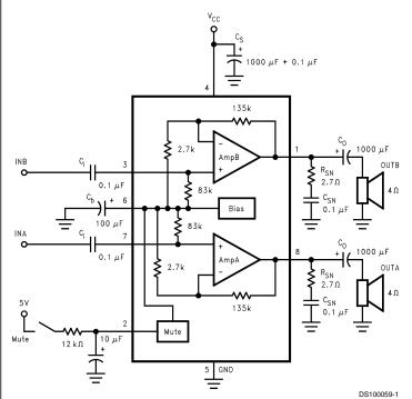
FIGURE 1. Typical Audio Amplifier Application Circuit
