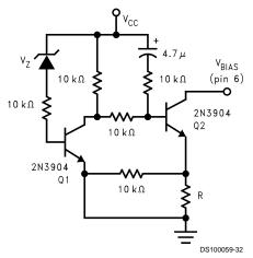
FIGURE 6. External Undervoltage Pull-Down
