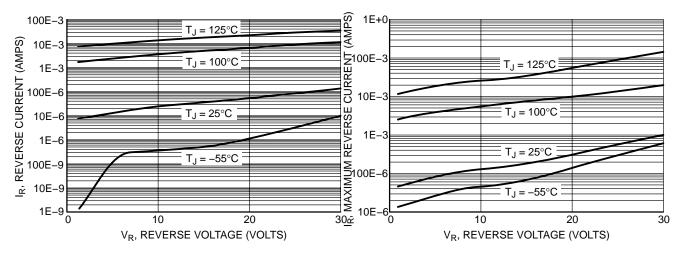
**Figure 3. Typical Reverse Current**
