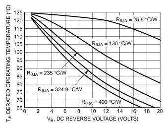
Figure 8. Typical Operating Temperature Derating
