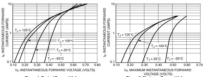
Figure 1. Typical Forward Voltage
