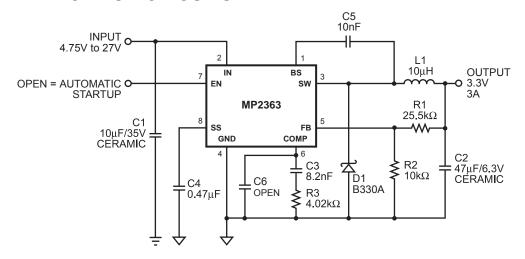
Figure 3—MP2363 for 3.3V Output with 47μF, 6.3V Ceramic Output Capacitor
