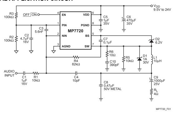
Figure 1—20W Mono Typical Application Circuit
