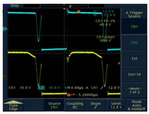
pic.1 secondary winding output and gate voltage of MOSFET waveform at discontinuous mode condition.
