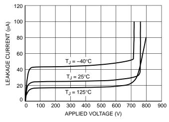
Figure 15. Power Switch and Startup Circuit Leakage Current versus Voltage
