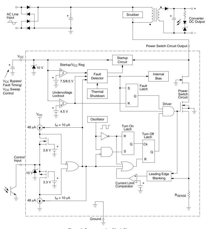
Figure 2. Representative Block Diagram
