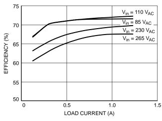
Figure 36. Converter Efficiency
