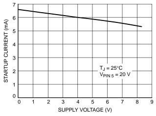
Figure 21. Startup Current versus Supply Voltage
