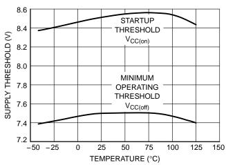
Figure 18. Supply Voltage Thresholds versus
