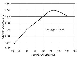
Figure 13. Control Input Upper Window Clamp
