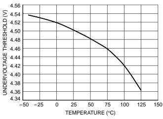
Figure 19. Undervoltage Lockout Threshold versus Temperature
