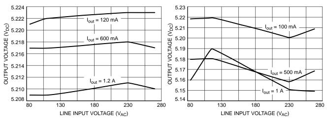
Figure 30. Converter Line Regulation
