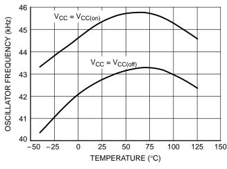
Figure 5. Oscillator Frequency (A Suffix) versus Temperature
