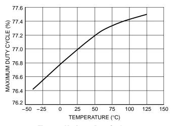
Figure 9. Maximum Duty Cycle versus Temperature
