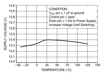
Figure 27. Supply Voltage versus Temperature
