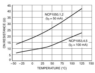
Figure 14. On Resistance versus Temperature
