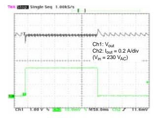
Figure 35. Charger Load Transient Response
