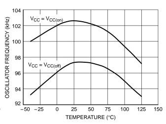
Figure 6. Oscillator Frequency (B Suffix) versus Temperature
