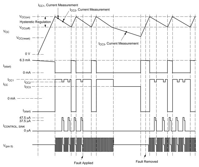
Figure 4. Non-Latching Fault Condition Timing Diagram
