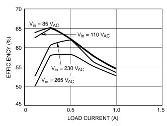
Figure 37. Charger Efficiency
