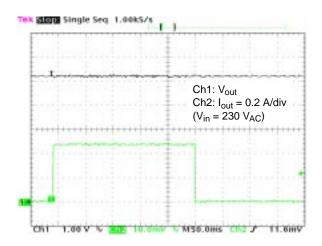
Figure 34. Converter Load Transient Response
