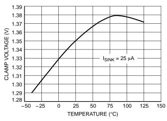
Figure 12. Control Input Lower Window Clamp Voltage versus Temperature
