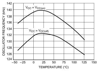
Figure 7. Oscillator Frequency (C Suffix) versus Temperature
