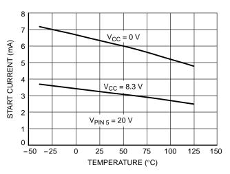
Figure 20. Start Current versus Temperature
