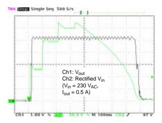
Figure 39. Charger On/Off Line Transient Response
