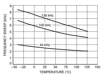
Figure 8. Frequency Sweep versus Temperature
