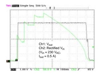
Figure 38. Converter On/Off Line Transient Response
