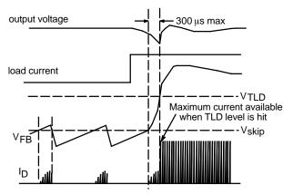
Figure 37. Transient Response from Standby
