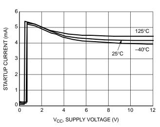
Figure 18. Startup Current vs. V<sub>CC</sub> Voltage
