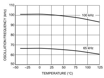
Figure 3. Oscillation Frequency vs.
