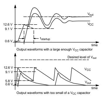
Figure 26. Different Startup Scenarios of the Circuits with Different V<sub>CC</sub> Capacitors
