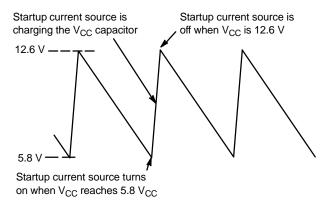
Figure 38. Latchoff V<sub>CC</sub> Timing Diagram
