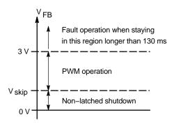
Figure 40. NCP1271 Operation Threshold
