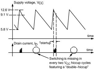
Figure 25. V<sub>CC</sub> Double Hiccup Operation in a Fault Condition
