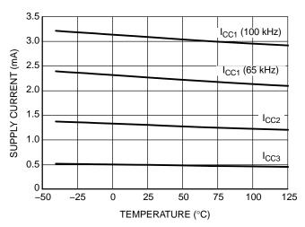
Figure 22. Supply Currents vs. Temperature
