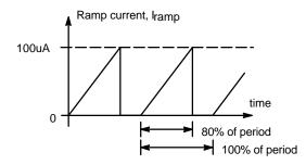
Figure 32. Internal Ramp Current Source
