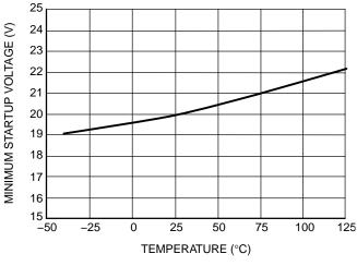
Figure 20. Minimum Startup Voltage vs. Temperature
