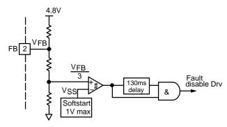
Figure 35. Block Diagram of Timer-Based Fault Detection
