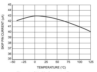
Figure 9. Default Skip Level vs. Temperature
