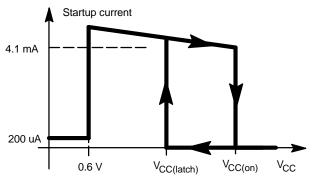
Figure 23. Startup Current at Various V<sub>CC</sub> Levels
