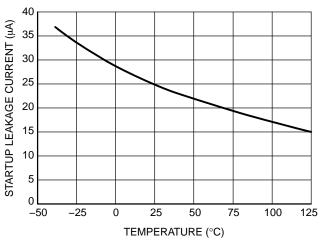
Figure 19. Startup Leakage Current vs. Temperature
