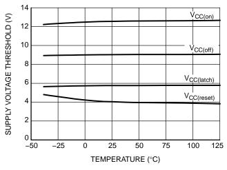
Figure 21. Supply Voltage Thresholds vs. Temperature
