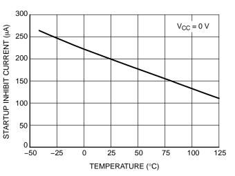
Figure 15. Startup Inhibit Voltage vs. Temperature
