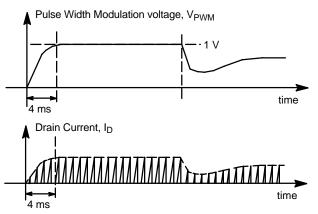
Figure 29. Soft-Start (Time = 0 at  $V_{CC} = V_{CC(on)}$ )
