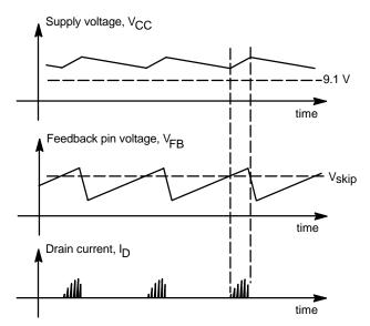
Figure 27. Timing Diagram of Standby Condition
