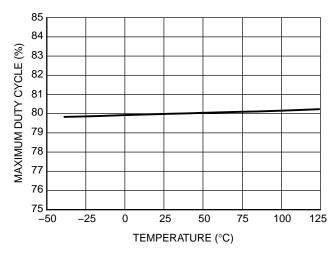
Figure 4. Maximum Duty Cycle vs. Temperature
