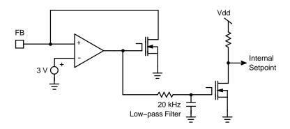
Figure 7. Internal Implementation of FB Pin
