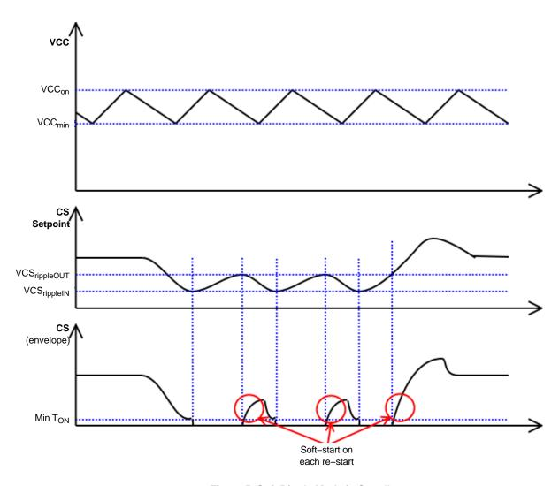
Figure 5. Soft Ripple Mode in Standby
