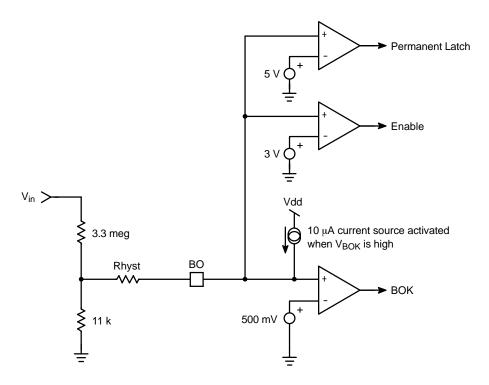
Figure 8. Internal Implementation of BO Pin
