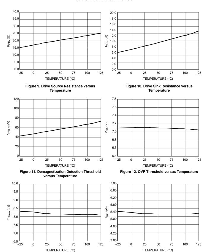
Figure 13. Minimum T<sub>OFF</sub> versus Temperature
