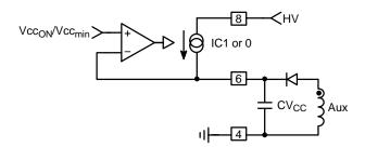
Figure 16. The Current Source Brings Vcc Above Vcc<sub>ON</sub> and Then Turns Off
