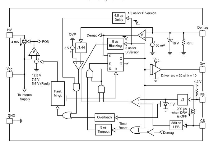
**Figure 2. Internal Circuit Architecture**
