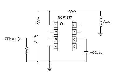
Figure 26. A simple transistor arrangement triggers the latchoff as soon as the temperature exceeds a given setpoint.
