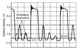
Figure 21. Core Reset Detection is Done through a Dedicated Auxiliary Winding Monitoring
