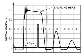
Figure 24. A Voltage Sample is Taken 4.5 μs
