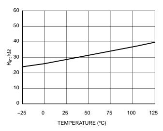
Figure 15. DMG Pin Internal Resistance versus Temperature
