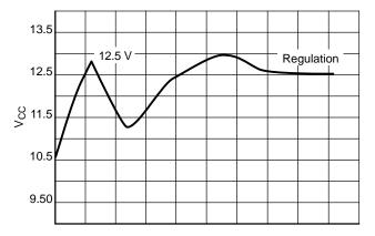
Figure 17. A Typical Startup Sequence for the NCP1377
