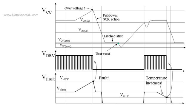
Figure 42. Overvoltage and Overtemperature Chronograms
