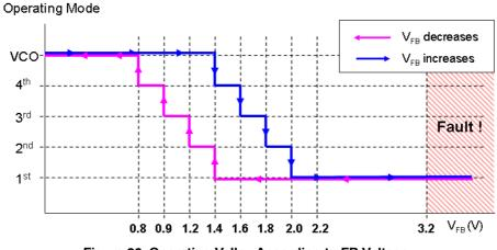
Figure 26. Operating Valley According to FB Voltage
