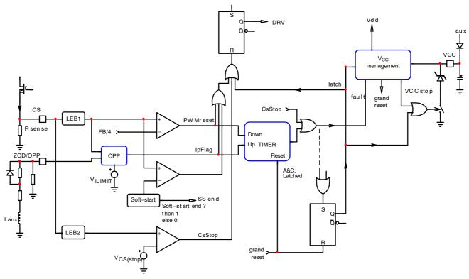
Figure 37. Overload Detection Schematic
