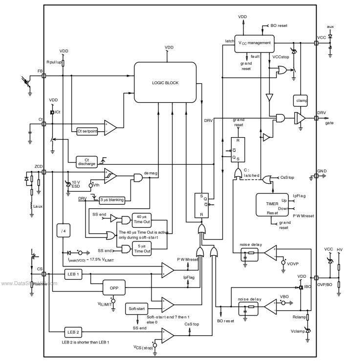
Figure 4. Internal Circuit Architecture for Versions C and D
