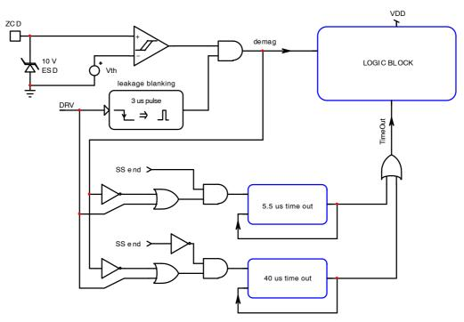
Figure 33. Time Out Circuit
