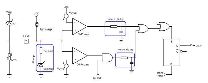
Figure 41. OVP/OTP Circuitry
