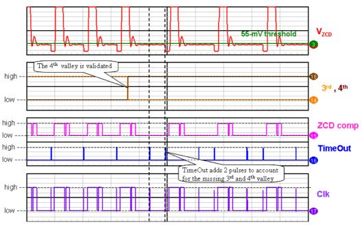
Figure 35. Time Out Case n°2: the 3<sup>rd</sup> and 4<sup>th</sup> Valley are Missing
