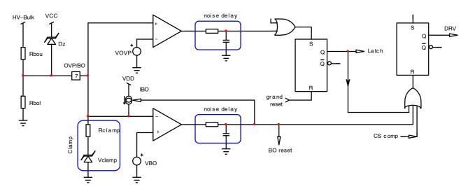
Figure 43. Brown-out and Overvoltage Protection
