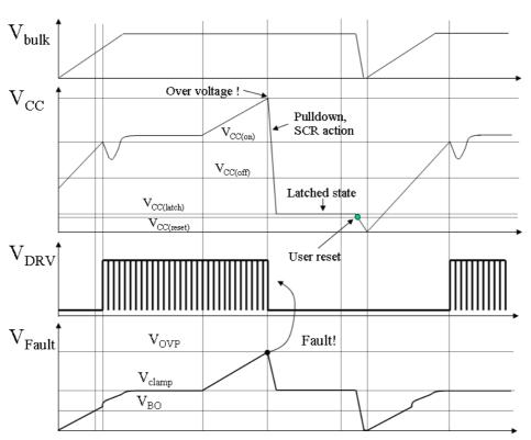
Figure 45. Operating Chronograms in Case of Overvoltage
