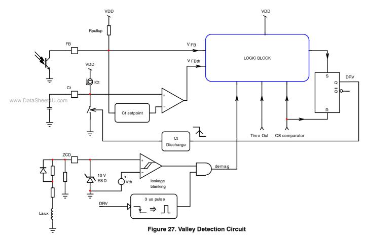
As the output load decreases (FB voltage decreases), the valleys are incremented from the first to the fourth. When the fourth valley is reached, if FB voltage further decreases below 0.8 V, the controller enters VCO mode.
