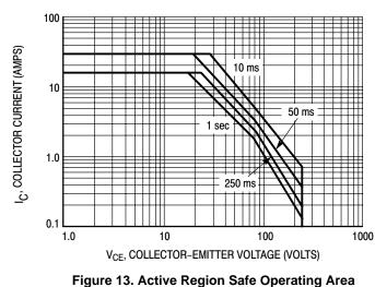
There are two limitations on the power handling ability of a transistor; average junction temperature and secondary breakdown. Safe operating area curves indicate I<sub>C</sub> - V<sub>CE</sub> limits of the transistor that must be observed for reliable operation; i.e., the transistor must not be subjected to greater dissipation than the curves indicate.
