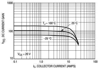
Figure 3. DC Current Gain, V<sub>CE</sub> = 20 V
