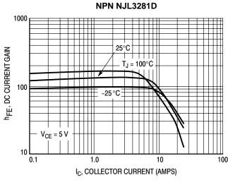
Figure 6. DC Current Gain, V<sub>CE</sub> = 5 V
