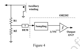
If the sampled plateau voltage exceeds the OVP trip level (3.75V), the controller stops all switching operations and enters into latch off mode.
