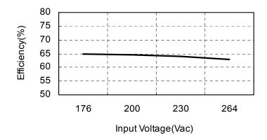
Figure 2. Efficiency @200mA load
