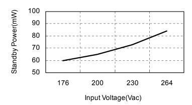
Figure 1. Standby input power
