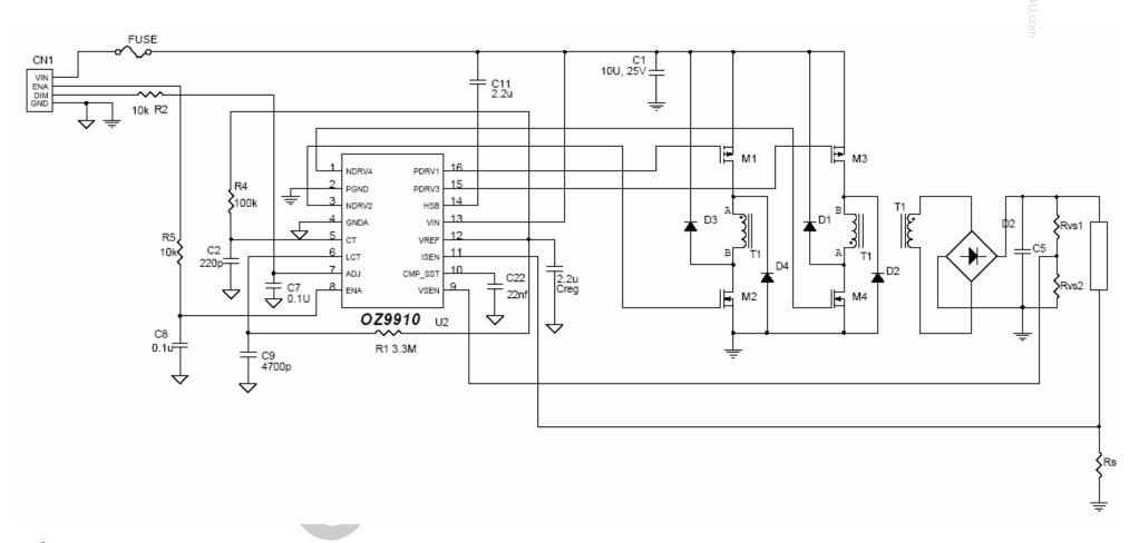
**Figure 3. Application Circuit for TWT**
