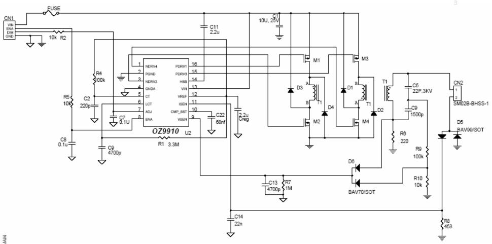
Figure 2. Application Circuit for CCFL
