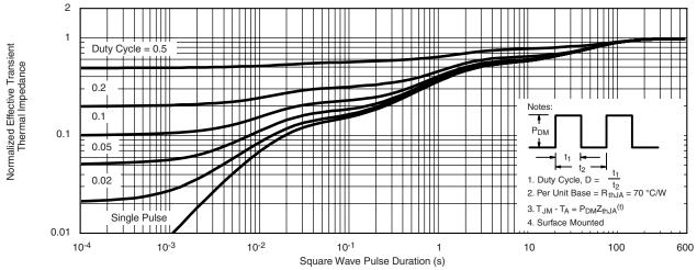
Normalized Thermal Transient Impedance, Junction-to-Ambient
