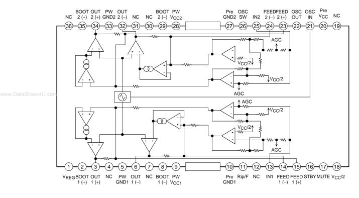
\*: Some of the functional blocks, circuits, or constants in the block diagram may be omitted or simplified for explanatory purpose.
