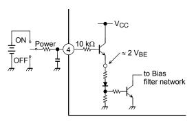
Figure 1 Setting Pin 4 High Turns on Power
