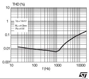
Figure 9. Distortion vs. frequency.
