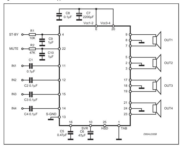
Figure 1: Standard Test and Application Circuit
