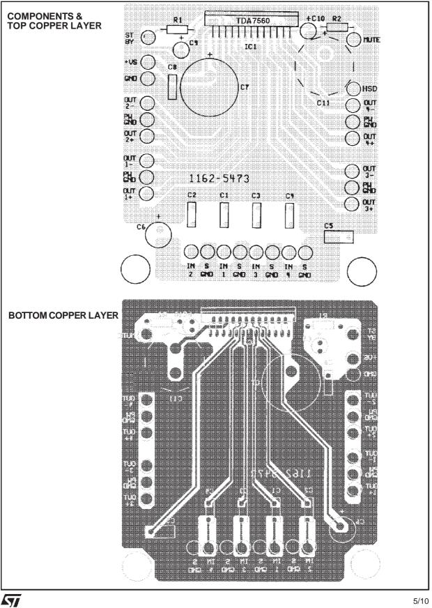
Figure 2: P.C.B. and component layout of the figure 1 (1:1 scale)
