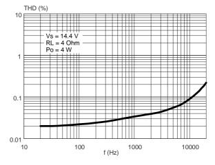
Figure 8. Distortion vs. Frequency (2W)
