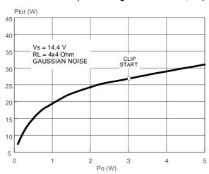
Figure 13. Power Dissipation vs. Average Ouput Power (Audio Program Simulation,  $2\Omega$ )
