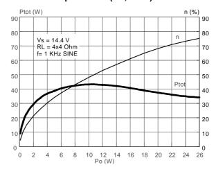
Figure 12. Power Dissipation vs. Average Ouput Power (Audio Program Simulation,  $4\Omega$ )
