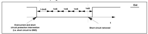
Figure 18. Restart timing with Diagnostic Enable (Permanent)
