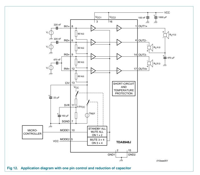
**Remark:** Because of switching inductive loads, the output voltage can rise beyond the maximum supply voltage of 28 V. At high supply voltages, it is recommended to use (Schottky) diodes to the supply voltage and ground.
