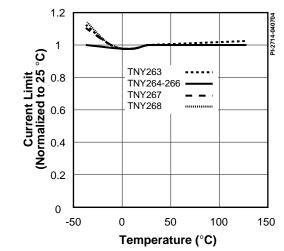
Figure 24. Current Limit vs. Temperature.
