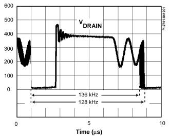
Figure 4. Frequency Jitter.
