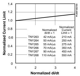
Figure 25. Current Limit vs. di/dt.
