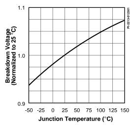
Figure 22. Breakdown vs. Temperature.
