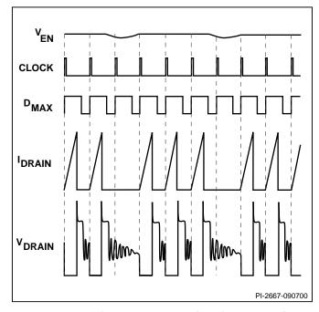
Figure 7. TinySwitch-II Operation at Moderately Heavy Loading.
