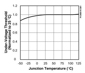
Figure 30. Undervoltage Threshold vs. Temperature.
