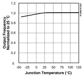
Figure 23. Frequency vs. Temperature.
