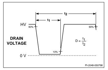
Figure 19. TinySwitch-II Duty Cycle Measurement.
