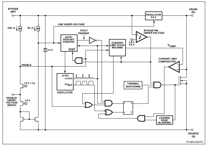
Figure 2. Functional Block Diagram.
