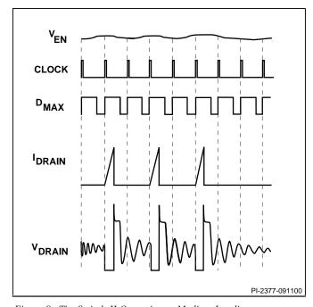
Figure 8. TinySwitch-II Operation at Medium Loading.
