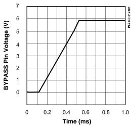
Figure 26. Bypass Pin Start-up Waveform.
