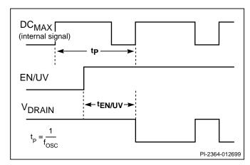
Figure 20. TinySwitch-II Output Enable Timing.
