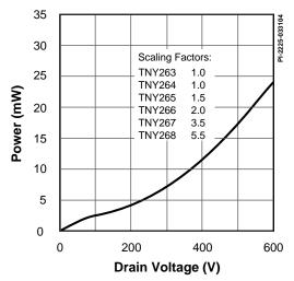
Figure 29. Drain Capacitance Power.
