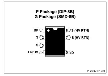
Figure 3. Pin Configuration.
