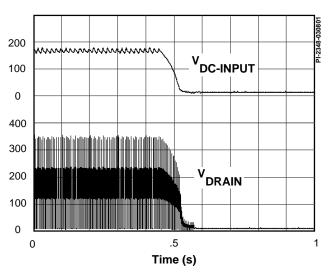
Figure 12. Normal Power-down Timing (without UV).
