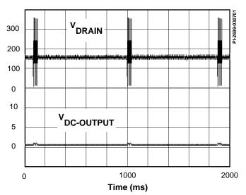
Figure 5. TinySwitch-II Auto-Restart Operation.
