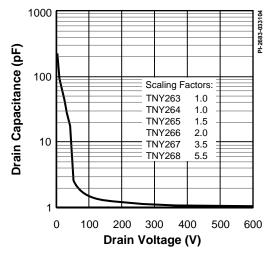
Figure 28.  $C_{oss}$  vs. Drain Voltage.
