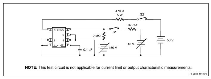
Figure 18. TinySwitch-II General Test Circuit.
