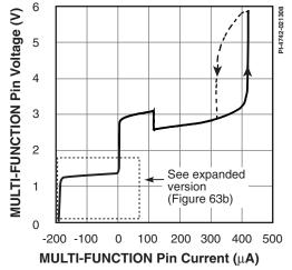
Figure 63a. MULTI-FUNCTION Pin Voltage vs. Current.
