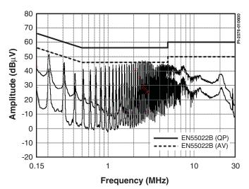
Figure 45a. Fixed Frequency Operation Without Jitter.
