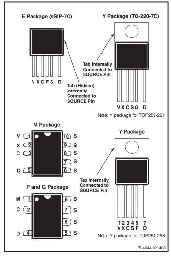
Figure 4. Pin Configuration (Top View).
