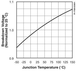
Figure 56. Breakdown Voltage vs. Temperature.
