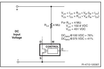
Figure 7. P/G Package Line Sense.
