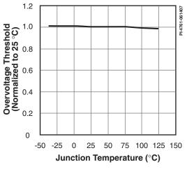
Figure 60. Overvoltage Threshold vs. Temperature.
