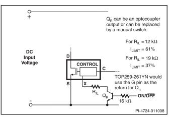
Figure 25. Active-on Remote ON/OFF with Externally Set Current Limit.
