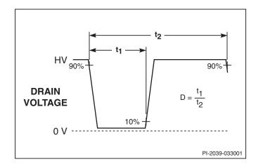
Figure 51. Duty Cycle Measurement.
