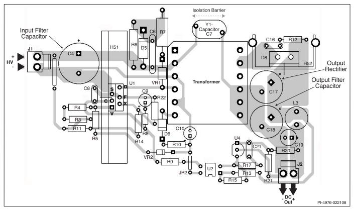
Figure 50b. Layout Considerations for TOPSwitch-HX Using E-Package and Operating at 132 KHz.
