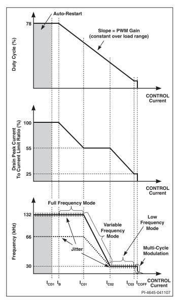
Figure 9. Control Pin Characteristics (Multi-Mode Operation).
