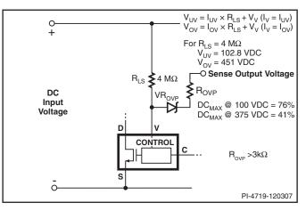
Figure 19. Line-Sensing for Undervoltage, Overvoltage, Line Feed-Forward and Hysteretic Output Overvoltage Protection.
