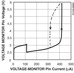
Figure 62a. LINE-SENSE Pin Voltage vs. Current.
