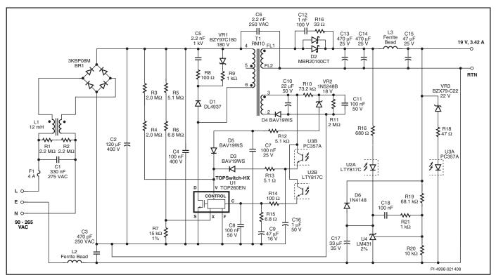
Figure 44. 65 W, 19 V Power Supply Using TOP260EN.
