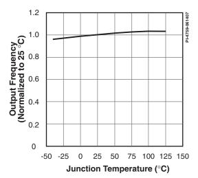
Figure 57. Frequency vs. Temperature.
