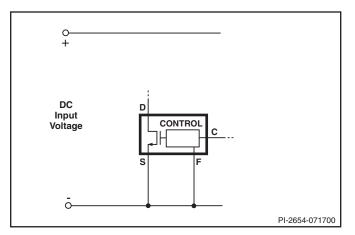
Figure 14. Full Frequency Operation (132 kHz).
