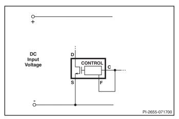
Figure 15. Half Frequency Operation (66 kHz).
