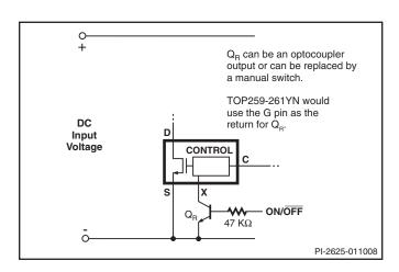
Figure 24. Active-on (Fail Safe) Remote ON/OFF.
