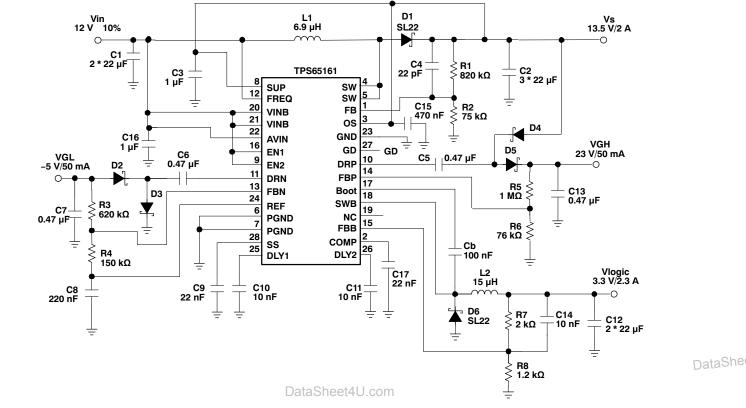
Figure 22. Standard 12-V to 13.5-V Conversion
