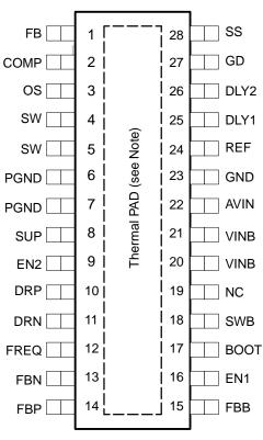
NOTE: The thermally enhanced PowerPAD<sup>™</sup> is connected to PGND.
