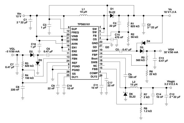
Figure 20. Standard 12-V to 18-V Conversion
