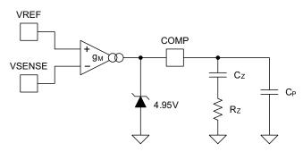
Figure 27. Transconductance Error Amplifier with Typical Compensation Network
