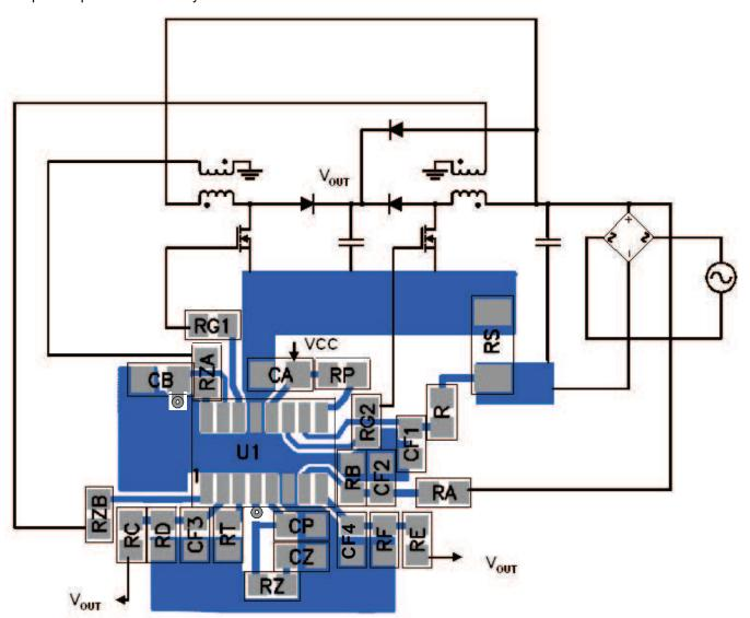
Figure 35. Recommended PCB Layout
