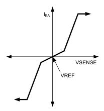
Figure 28. Basic Voltage-Error Amplifier Transconductance Curve
