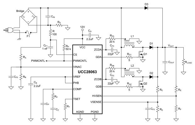
Figure 34. Typical Interleaved Transition-Mode PFC Pre-Regulator
