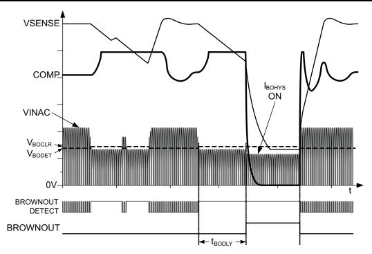
Figure 31. AC-Line Brownout Timing with Illustrative System Behavior
