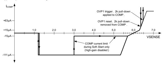
Figure 29. Expanded COMP Output Current Curve
