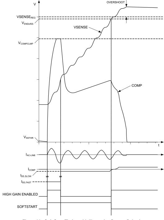
Figure 30. Soft-Start Timing with Illustrative System Behavior
